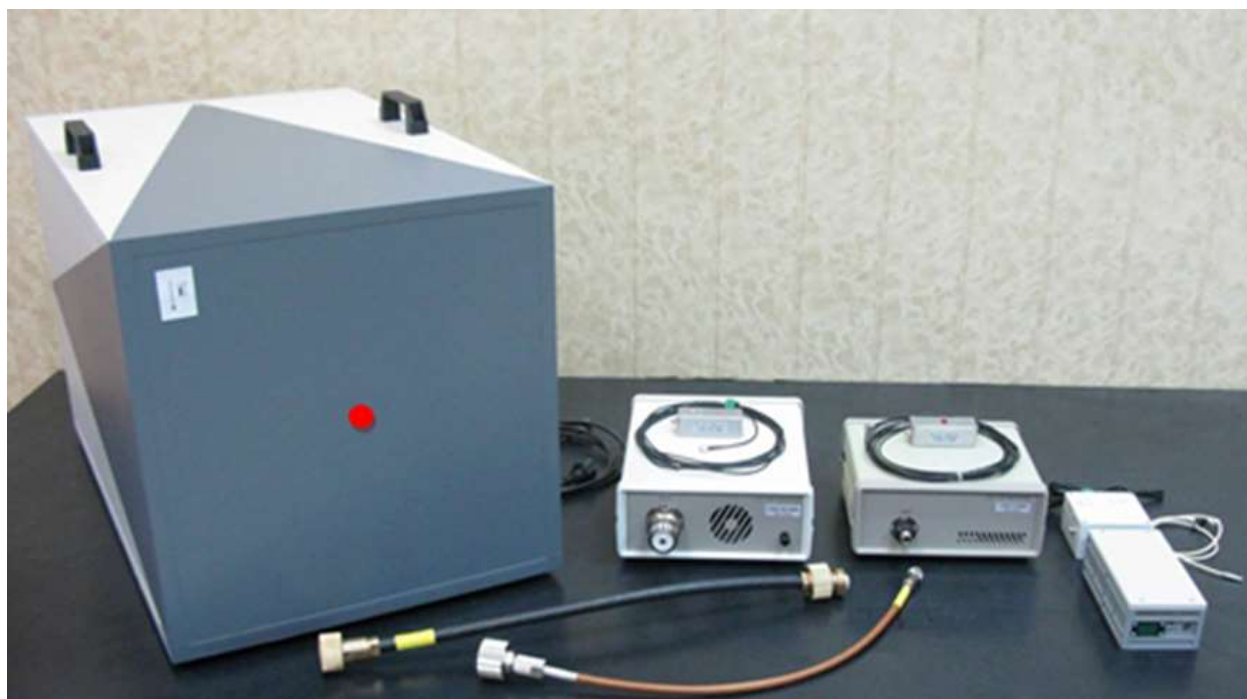
Fig. 1. Mobile complex for testing of equipment immunity to UWB EMP
