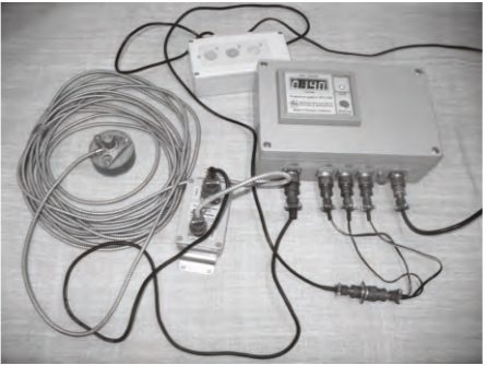
Single-channel vibration meter with vibration shutdown function
