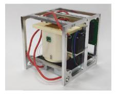
The micromotor was developed jointly with ITMO University (Russia) within the framework of the Union State Program "Technology-SG". Designed to move, maneuver and maintain the altitude of low Earth orbit for small spacecraft of the CubeSat format.
