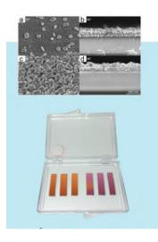
A line of photonic sensors has been developed that, depending on the morphology of the sensitive area, make it possible to detect and study the structure of molecules, including biomarkers of diseases, and with high accuracy analyze biological fluids and sanitary-epidemiological washings using Raman spectroscopy.
