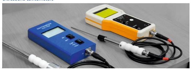
At the University's own production base the spectral-acoustic cavitation indicator and portable cavitometer are manufactured, which are designed for measuring and controlling cavitation activity and surpass foreign analogues in terms of functionality.
