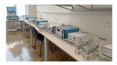
These are complexes of microwave test and measurement equipment and special software designed to calibrate microwave measurement devices (power meters and attenuators) widely used in radio astronomy, radio spectroscopy, radar, communications, applied metrology, etc.
