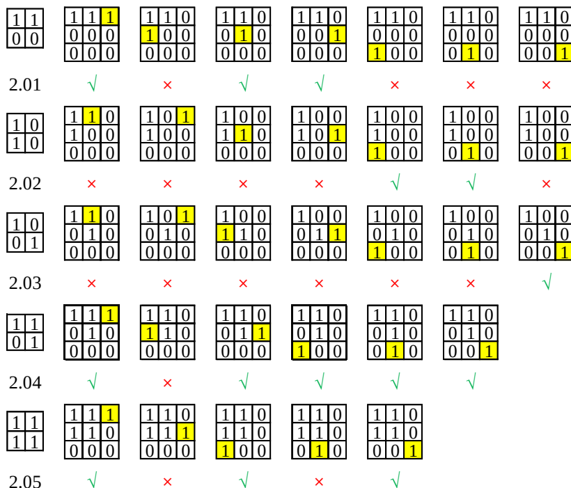
Fig. 2. Procedure of extending basic set of size 2 \times 2 to pattern errors of all size 3 \times 3 and the procedure of reducing error patterns of order 3 to basis set of order t = 3:5
