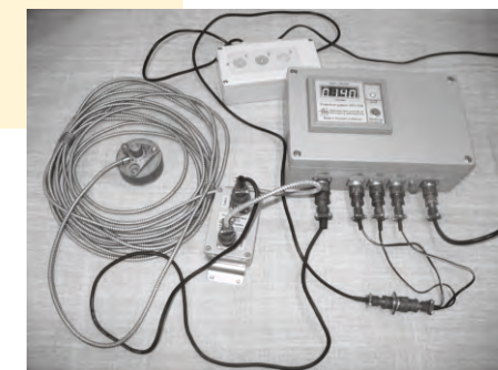
Single-channel vibration meter with safety shutdown on vibration function
