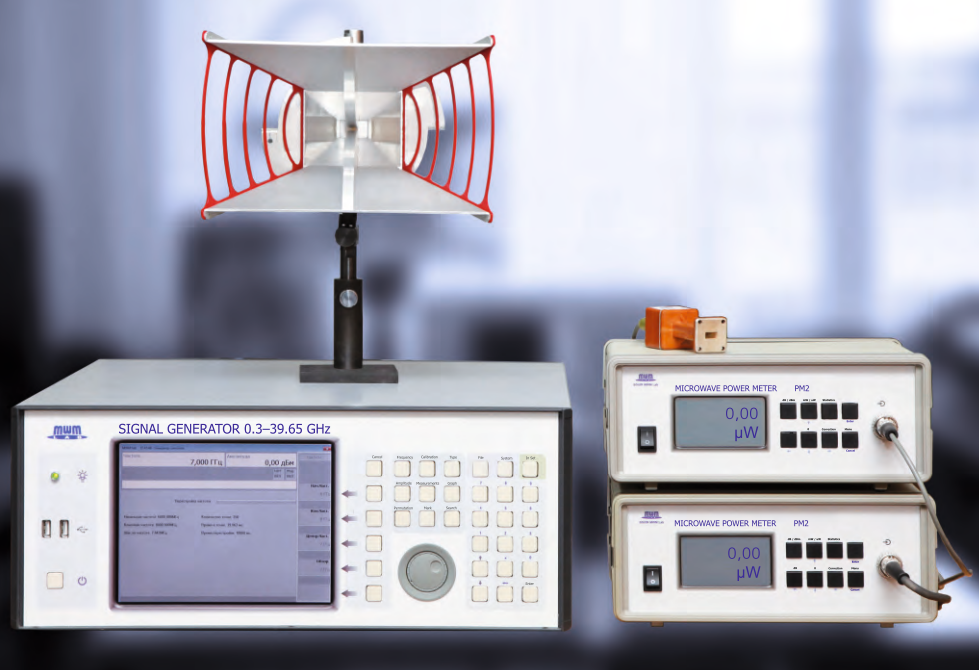
Emitting part of the of power flux density measurement standard unit with automatic adjustment
